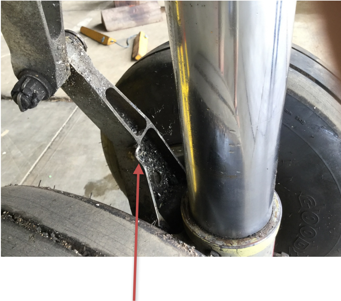
Fig.3 DEFLECTION THE TORQUE LINK ASSY
