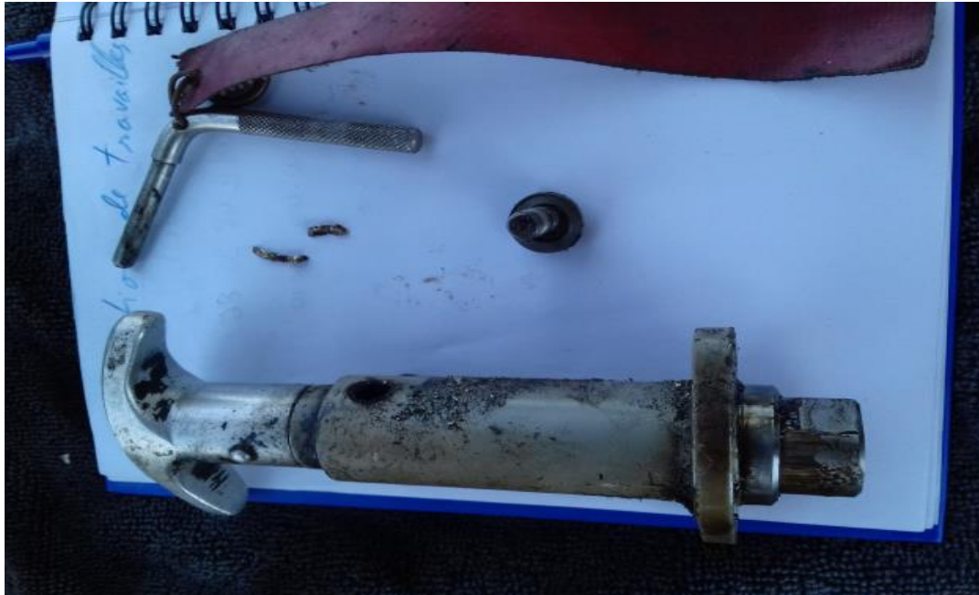
Fig.4 Safety Pin (for towing) and NLG Steering Coupling Mechanism
